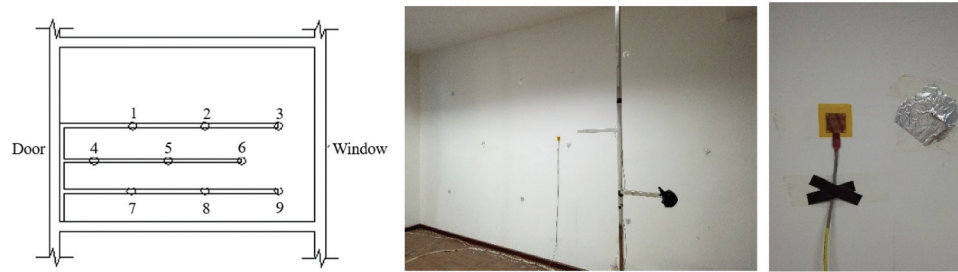
Figure 5. Schematic diagram of the temperature and heat flux measurement points distribution of the exterior wall and the interior partition.
