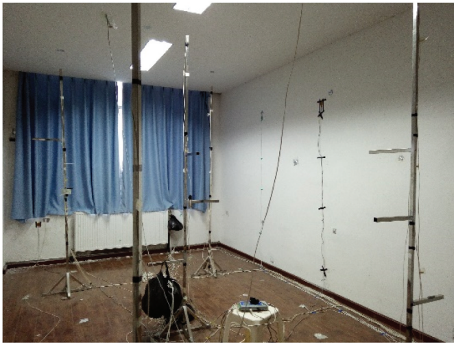
Figure 6. Schematic diagram of the temperature measurement points in the working space.
